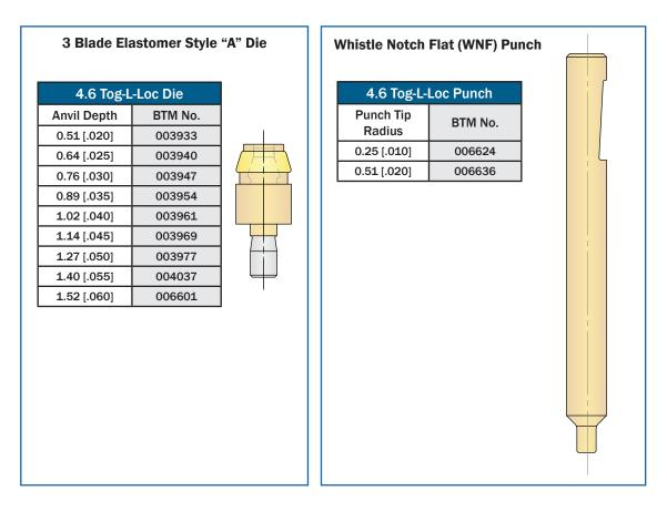
The correct Anvil Depth and Punch Tip Radius are determined through testing and/or by surrogate joint data at BTM. Contact a BTM sales application engineer to determine the correct tooling for your application.
